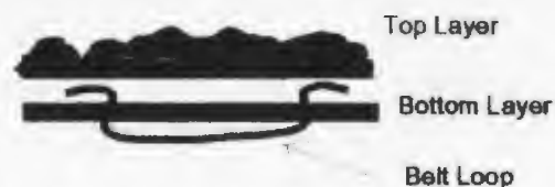
Figure 2. BUCKLE END VIEW
